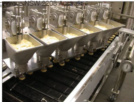
Above; Belshaw Vacumatic - deposits ring donuts directly to automatic proofer
