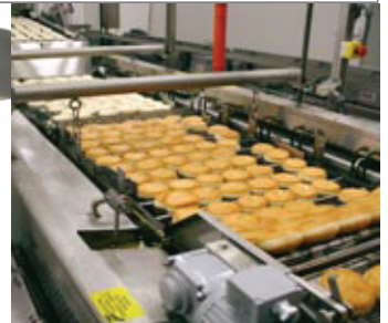
Century C10-24 — 10 ft. fryer, 6 standard donuts per pocket, shown frying raised donuts. Gas and electric models available. Conveyor hoist is standard. (Hood optional)
