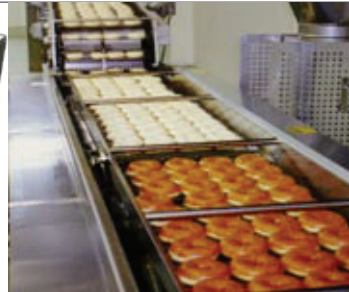
Century C6-24 — 6 ft. fryer, 6 standard donuts per pocket, shown at right with MDDRF-6 cake donut depositor. C6-24 is a gas-only fryer.
